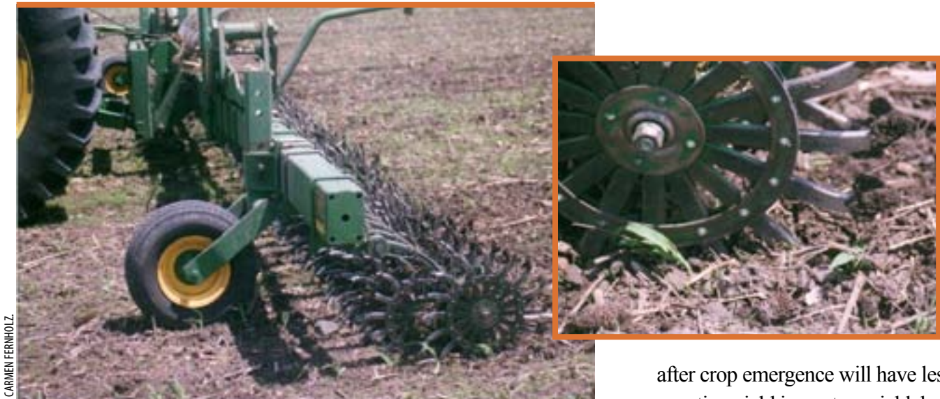
Figure 6-7. The rotary hoe has an operating depth of one inch or more.
