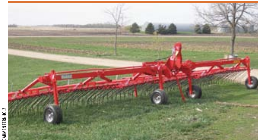
Figure 6-9. Flex-tine weeder. This tool is becoming more prevalent among organic producers in the Upper Midwest.
